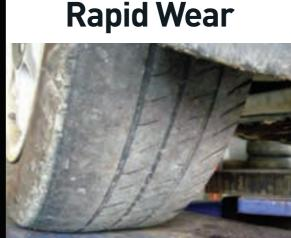
Misalignment(Toe)Insufficient tire rotation - Improper tire application **Heel & Toe Wear**
